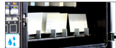
Condensation water test
