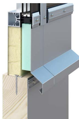
Vertical installation on wooden upstand
